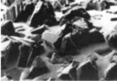
Coating of a single layer electroplated diamond grinding wheel (new).
